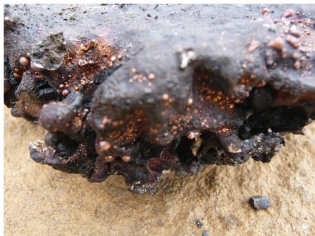
Figure 18. A slag cake with copper prills formed during Experiment 6A, Pločnik, Serbia in 2013 (photo: Simon Timberlake).
