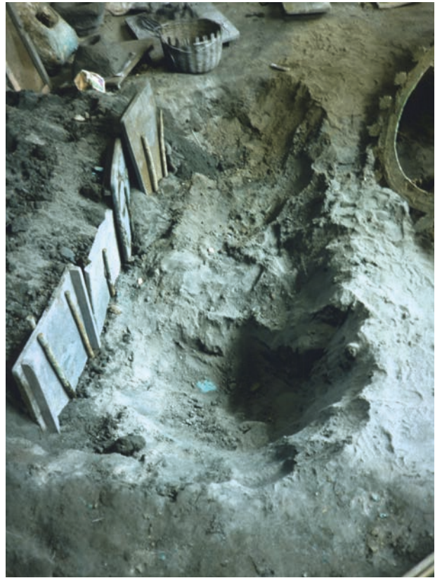
Fig. 13. The shallow casting pit in which the Shiva Nataraja (Fig. 12) was cast, lying face down at a slight angle (photo: P.T. Craddock).
