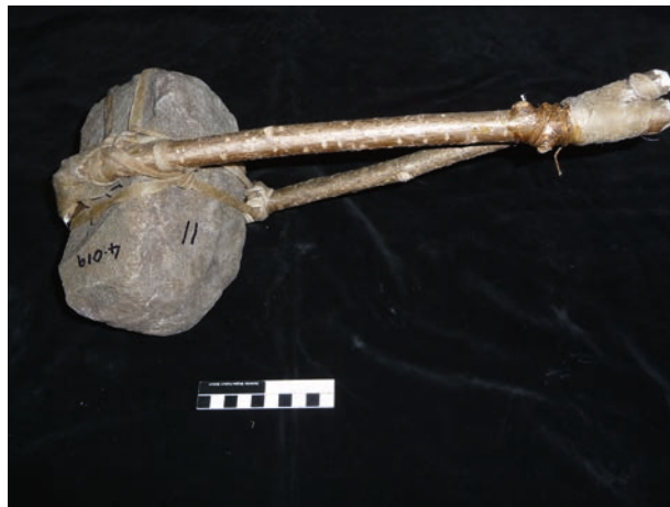
Fig 4. 'Chuquicamata-type' experimental mining hammer used at Sakdrisi Mine in 2011 (photo: Deutsches Bergbau-Museum Bochum).
