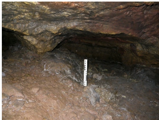
Fig. 3. Fireset working in the Canopa of Busa del Pomar (photo: M. Straßburger).
