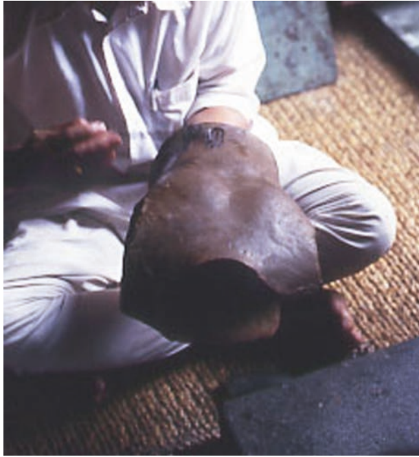
Fig. 7. Shaping the wax torso of a large statuette by the direct process, note the core has not yet been added. (Patan, 1987) (photo: P.T. Craddock).
