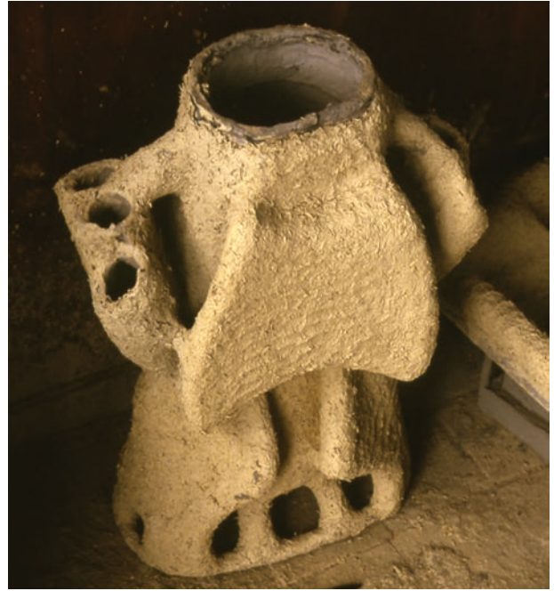
Fig. 8. Wax lower torso of deity after the application of the first layer of moulding clay by dipping and subsequent addition of outer layer of coarse clay and straw. Note the moulding is complete before the addition of the core, typical of the indirect process rather than direct castings (photo: P.T. Craddock).
