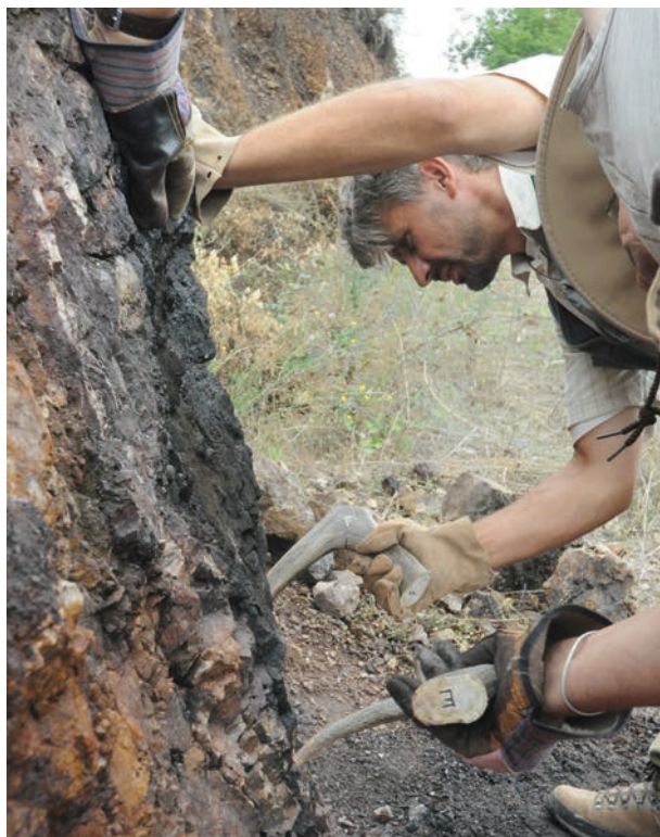
Fig. 7. The use of antler picks to remove a fireset quartz vein at the experimental mining site at Sakdrisi Mine in 2013 (photo: Deutsches Bergbau-Museum Bochum).
