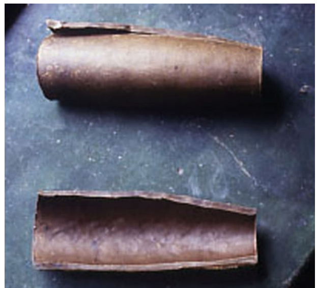
Fig. 9. Two sections of wax shaped by different processes, direct and indirect moulding. The upper sheet has been bent directly into a cylinder by hand, and there is just the one seam; the lower piece has been moulded indirectly by pressing the wax into a negative mould and to complete the cylinder; another piece will be required leaving two seams when joined (photo: P.T. Craddock).
