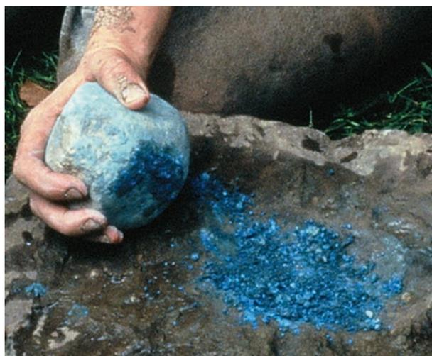
Figure 16. Azurite nodules as a copper ore from Engine Vein Mine, Alderley Edge, being prepared for smelting in 1997 (photo: Simon Timberlake).
