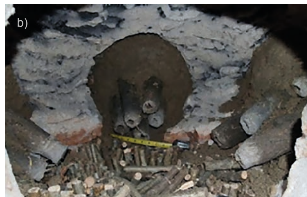
Fig. 14. Experimental iron smelting (a). Reconstruction of an African iron smelting furnace. The large nozzles are located directly in the specially manufactured furnace opening, which can be opened by any trip without destroying large parts of the furnace. Reaction chamber (b) of the upper iron smelting furnace (Source images a and b: http://warehamforgeblog.blogspot.de/2011/03/heat-under-africa.html . Full and complete copyrights: © Darrell Markewitz). The nozzles are directed at different angles to the melt. This feature corresponds to the different angles of the slagging at the nozzles from Tinma and Faynan (Rothenberg, 1990; Hauptmann, 2007; Al-Shorman, 2009; Ben-Yosef, 2010).
