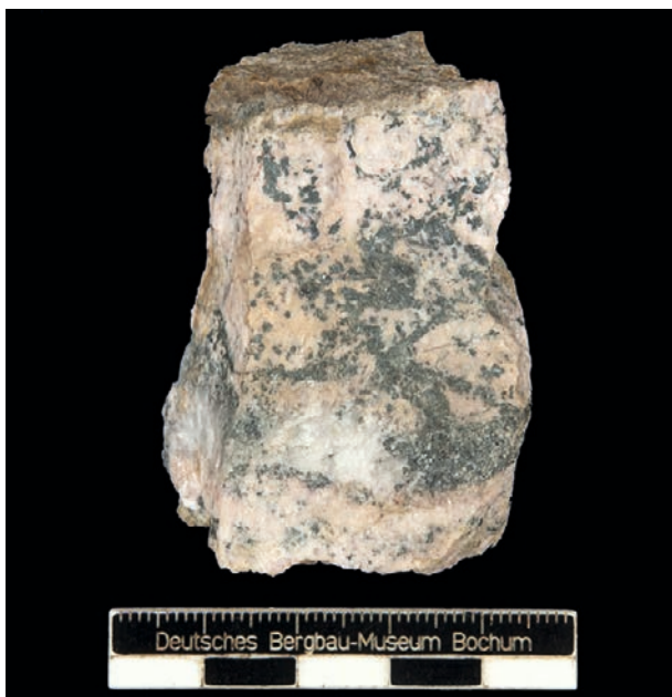
Fig. 2: Silver ore from Freiberg, Saxony (Beschert Glück). The dark areas are primarily the mineral acanthite (DBM Mineral Collection, Photo: S. Merkel).
