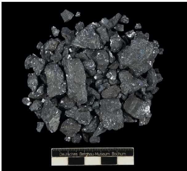
Fig. 1: Argentiferous galena from the Czech Republic. This galena was roasted, smelted and the silver was purified using analytical cupellation. The silver content of the smelted lead is 0.7 % (Photo: S. Merkel).
