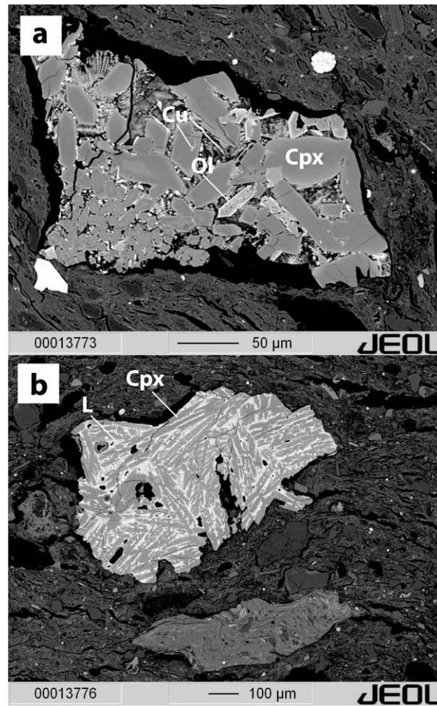
Fig. 7: Backscatter electron (BSE) images of slag fragments from the cemetery St. Leonhard (a: sample SL3; b: sample SL4). (a): slag fragment with the mineral assemblage clinopyroxene (Cpx) + olivine (Ol). Rarely clinopyroxene contains very tiny Cu-droplets (sample SL3). (b): slag-fragment with the mineral assemblage clinopyroxene (Cpx) + glass (L). Directly below a quartzphyllite temper fragment can be seen (sample SL4).
