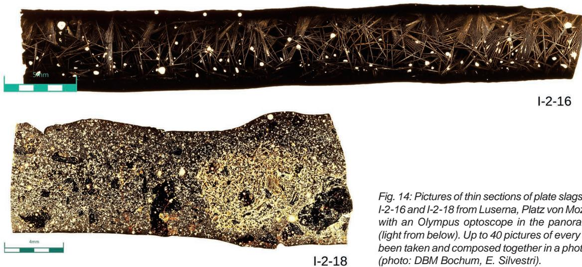
Fig. 14: Pictures of thin sections of plate slags (samples I-2-16 and I-2-18 from Luserna, Platz von Mozze) taken with an Olympus optoscope in the panorama mode (light from below). Up to 40 pictures of every slag have been taken and composed together in a photo mosaic; (photo: DBM Bochum, E. Silvestri).
