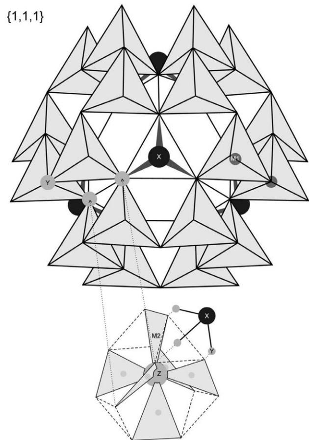
Fig. 2: Schematic illustration of the fahlore-group mineral structure according to Johnson et al. (1988). The chemical formula is  ${}^{IV}M(1)_6{}^{III}M(2)_6[{}^{III}X^{IV}Y_3]_4{}^{VI}Z$ .  $M(1) = Cu, Fe, Zn, Hg$ ;  $M(2) = Cu, Ag$ ;  $X = As, Sb, Bi$ ;  $Y = S$ ;  $Z = S, Se$ .
