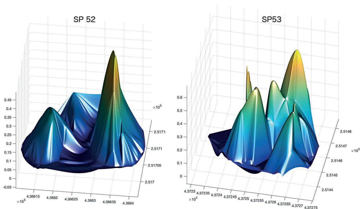
Fig 6: Examples of the 3-dimensional model of the slag heap used for the calculation of their volume. X and Y axes give the coordinates of the slag heap while the z axis presents its thickness in meters. The model is not a reconstruction of the actual 3D shape of the slag heap, but rather its thickness. The model was generated in MatLAB using a cubic interpolation (graphics: E. Hanning).
