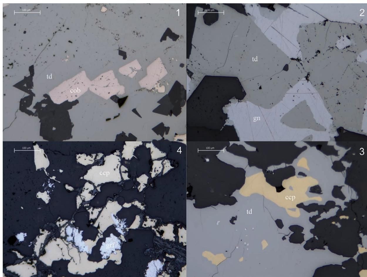
Fig. 7: Polished sections of ore samples. (1) Tetrahedrite (td) and cobaltite (cob), Rotenstein/Serfaus. (2) Tetrahedrite and galena (gn), Wildgrube/Oberberg. (3) Tetrahedrite and chalcopyrite (ccp), Knappenhäusl/Landeck. (4) Chalcopyrite and gersdorffite (grf), Großmutzkopf/Nauders.
