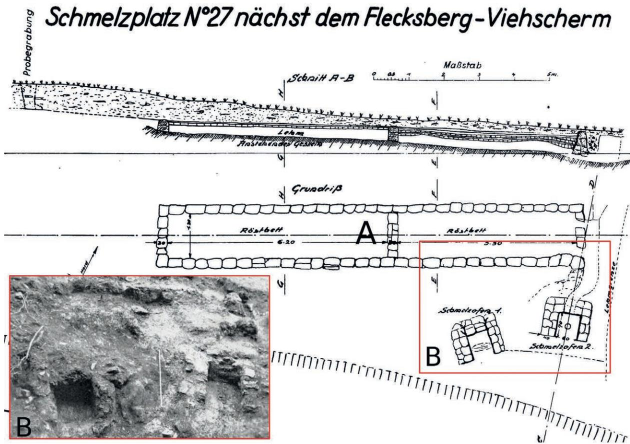
Fig 3: Drawing and photograph of a “typical” smelting site with roasting bed (A) and smelting furnaces (B and photo insert). Modified after Zschocke & Preuschen, 1932, pl. III and V.
