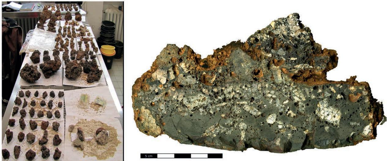
Fig 7. Left: selection of slag pieces in the slag heap sample. Right: Section through a larger piece of slag. Unmelted pieces of ore and gangue material are clearly visible as white inclusions in the slag.
