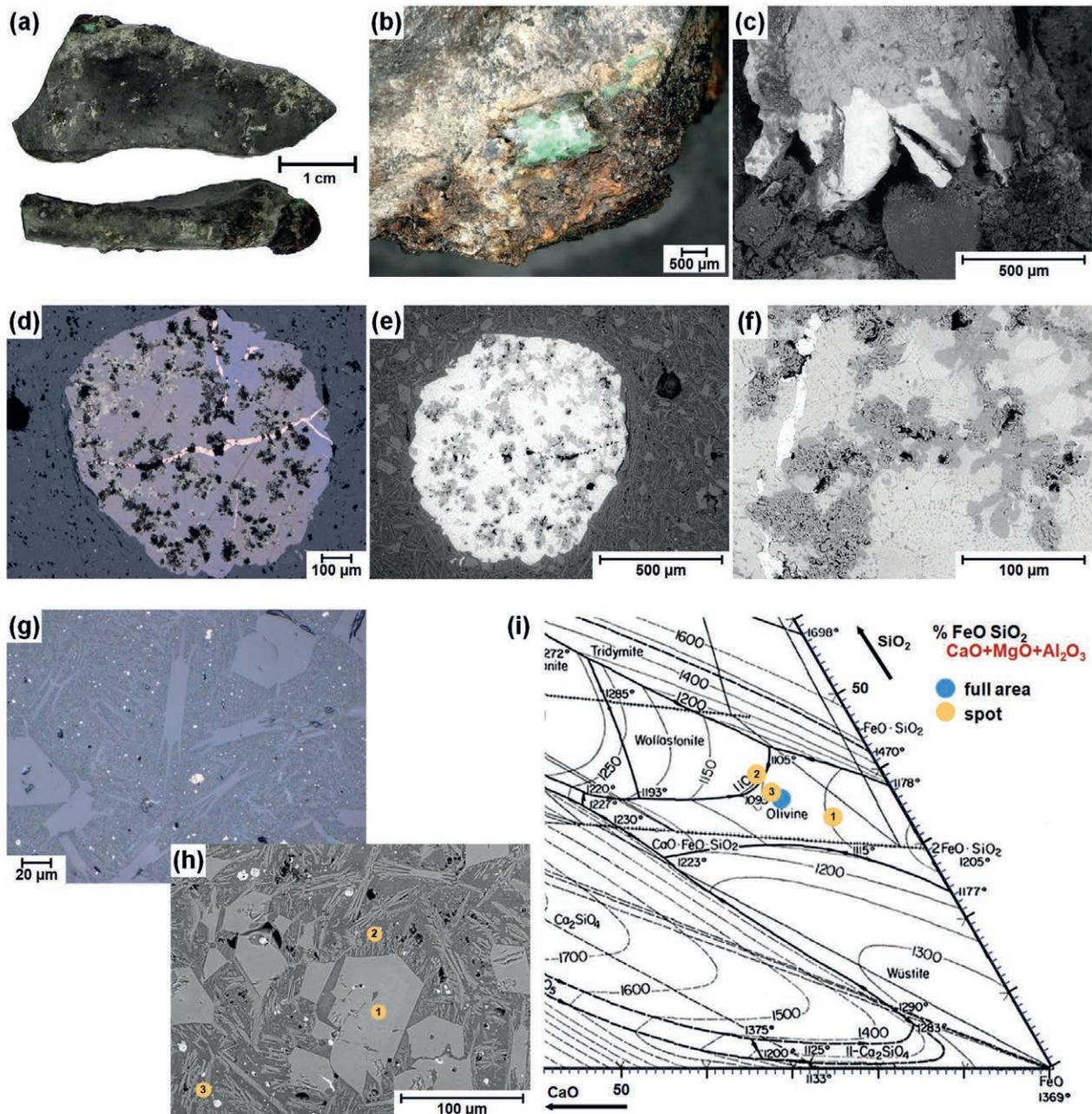
Fig. 5: Platy slag from Prigglitz-Gasteil (Pr 1896); (a) front and side view; (b) surface with Sn rich particle (3D-OM); (c) Sn rich particle in SEM); (d) copper rich inclusions (LOM); (e, f) SEM-BSE pictures of the Cu-rich inclusion; (g) slag microstructure in LOM; (h) SEM picture with indicated spots for EDX measurements; (i) phase diagram showing the elemental composition of the EDX measurements shown in (h).
