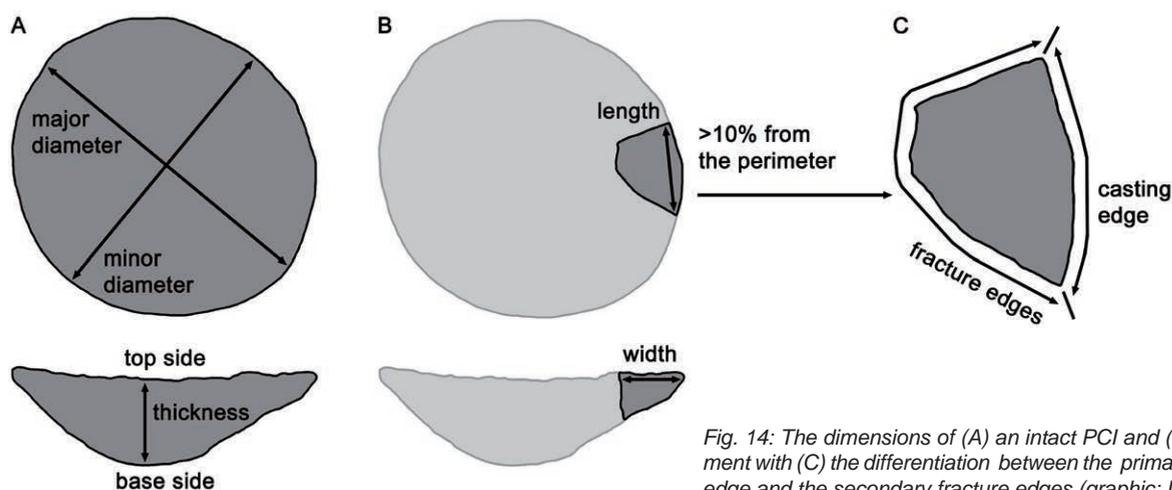
Fig. 14: The dimensions of (A) an intact PCI and (B) a fragment with (C) the differentiation between the primary casting edge and the secondary fracture edges (graphic: D. Modl).
