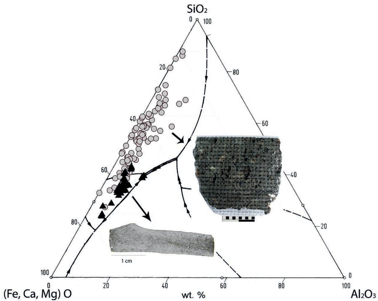
Fig. 17: Plots of the main oxide constituents in the phase diagram  $\text{SiO}_2 - \text{FeO} (+\text{CaO}+\text{MgO}) - \text{Al}_2\text{O}_3$  of plane scans performed on a slag cake (see Figure 12) and various plate slags. Ca. 100 spots were analysed on the slag cake, and 55 in thin sections of plate slags. Methods: pXRF (Niton XL3t), SEM (Zeiss Supra 40 VP). Note development from  $\text{SiO}_2$ -rich (unmelted) compositions to low melting subareas in the slag cake.
