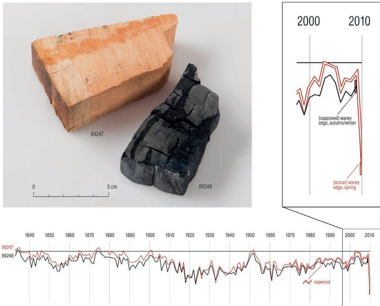
Fig. 3: Charcoal experiment. Recent alpine larch sample, charred and uncharred fragments and the correlation of both series. Values: Gleichläufigkeit 81.3,  $t$ -value after Hollstein 10.0 (graphic ADG).
