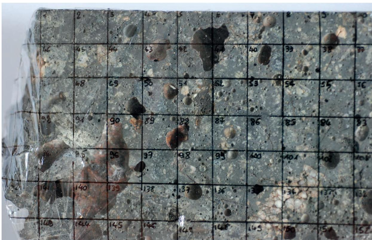
Fig. 12: Luserna, slag cake. The slag cake has been cut in two parts, to demonstrate the heterogeneous texture of this type of slag. Squares of 1 cm have been drawn on the surface, with the help of a transparent plastic foil. The image shows that relics of highly refractive, light minerals (mm- to cm-sized) are distributed throughout the cake. See Figure 17 for the chemical composition of the slag in the different squares (photo: DBM Bochum, E. Silvestri).
