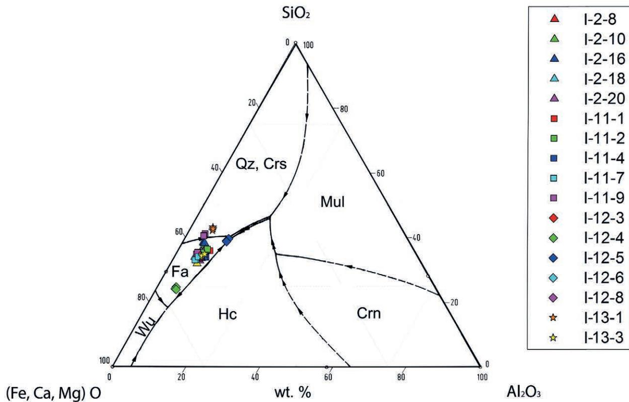
Fig. 13: Phase diagram  $\text{FeO} - \text{Al}_2\text{O}_3 - \text{SiO}_2$  (after Osborn & Muan, 1964) showing the bulk composition of plate slag samples from various slag heaps in the Trentino (1 Italy, 2 Luserna, 11 Transacqua, 12 Segonzano, 13 Malga Pontara), and sample number. Note that lower MgO and CaO contents were added to FeO.
