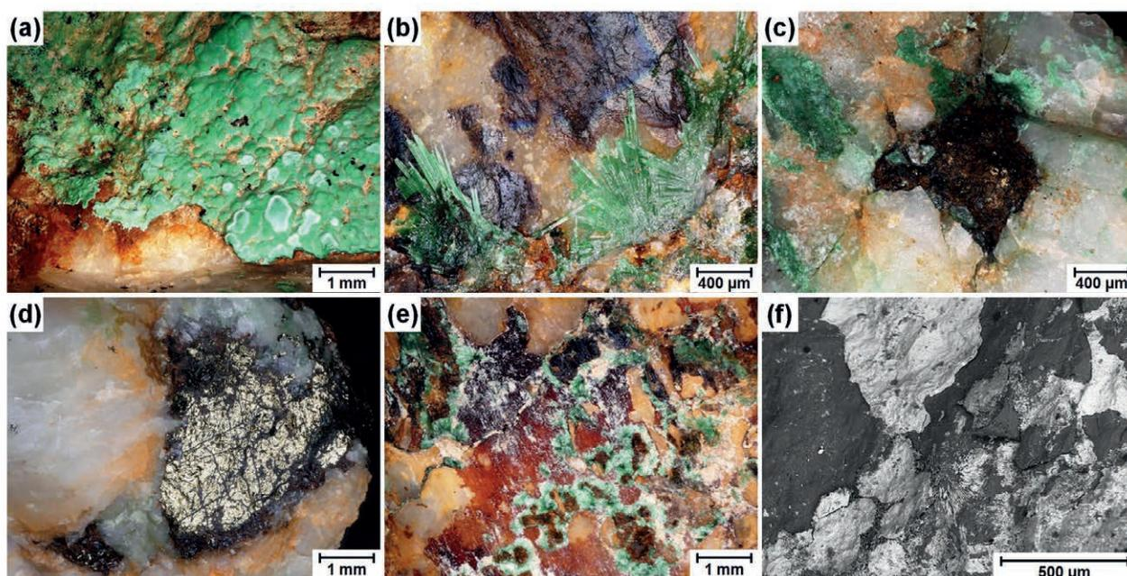
Fig. 2: Ore samples from Priggilitz-Gasteil Cu I in 3D-OM; (a) nodular malachite and quartz; (b) needle-like malachite; (c) limonite inclusion, (d) chalcopyrite in quartz; (e) mixture of malachite, cuprite and limonite; (f) SEM-BSE, cupreous regions are bright.
