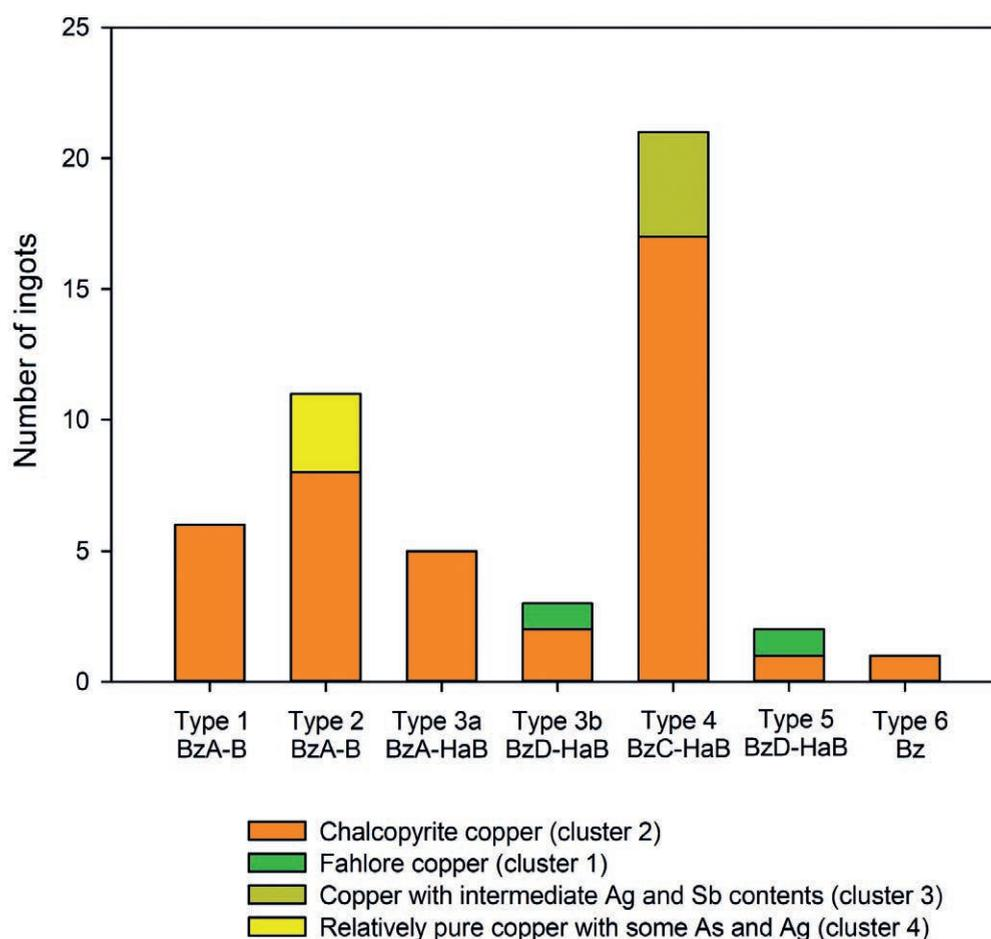
Fig. 7: Number of ingots of the different types analysed. The total number of analyses is larger, but many fragments could not be assigned to a certain type. Most ingots consist of chalcopyrite copper. Ingots made of fahlore copper or “diluted fahlore copper” are rare and occur only in the later periods. (© CEZA, Joachim Lutz).
