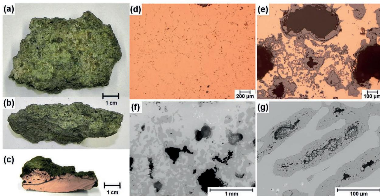
Fig. 4: Black copper lump Prigglitz Gastell Cu I; (a) front view; (b) side view; (c) cross section; (d) homogeneous copper with  $Cu_2S$  inclusions (LOM); (e) inhomogeneous region containing holes, sulfides and oxides (LOM); (f, g) SEM images showing the inclusions in metallic copper.
