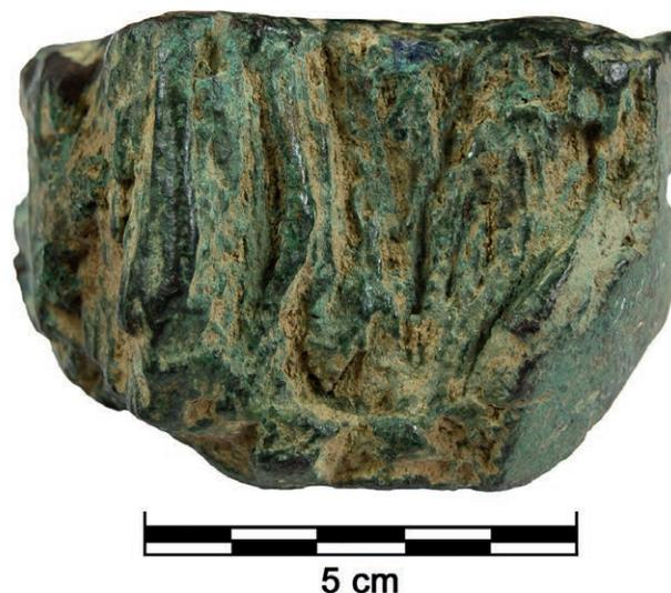
Fig. 25: Fragmented PCI with good visible columnar grains and hammer marks on the fracture surfaces from a hoard (HaA1) near Lannach, southwest of Graz, Styria (photo: D. Modl).
