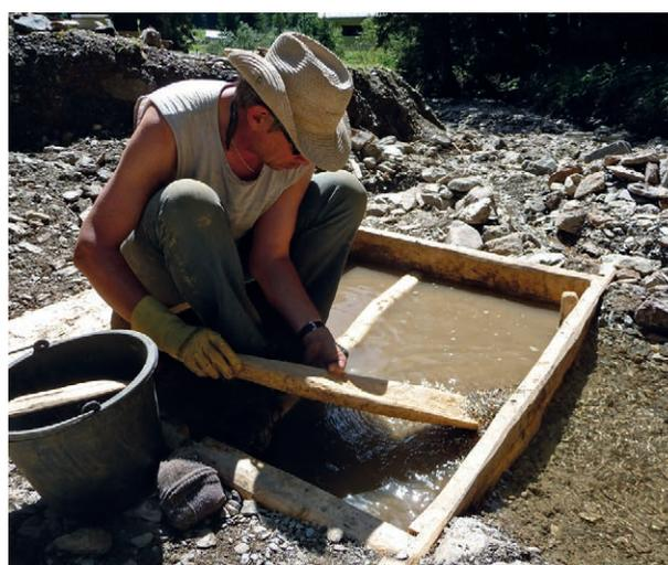
Fig. 6: Using the box as a buddle with a facsimile wooden shovel. August 2012 (photo: DBM).
