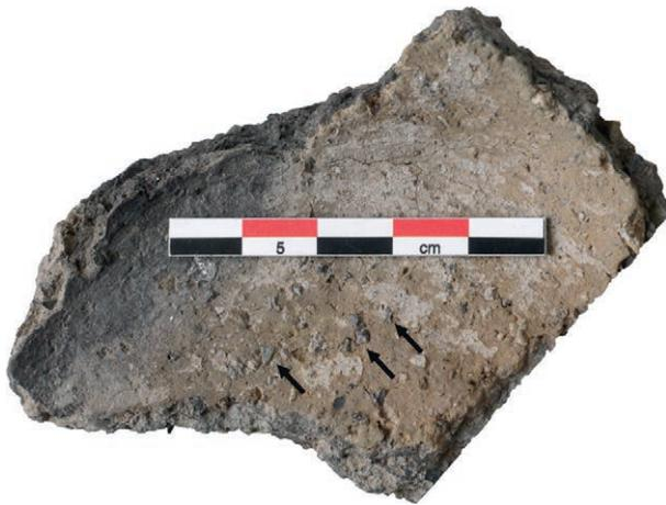
Fig. 4: Photograph of a ceramic fragment with visible slag-temper fragments on the surface (dark aggregates indicated with black arrows) from Kundl-Wimpassinger (sample W1).
