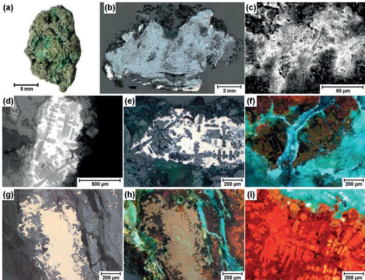
Fig. 6: Bronze droplet (P1778); (a) front view; (b) metallographic cross section (LOM); (c) droplet surface (SEM-BSE); (d – f) microstructure near the droplet surface (SEM and LOM); (g – i) cross section near the droplet center (LOM) – (g) metallic bronze (h) same location in LOM with polarized light (i) corroded bronze in the center of the droplet.
