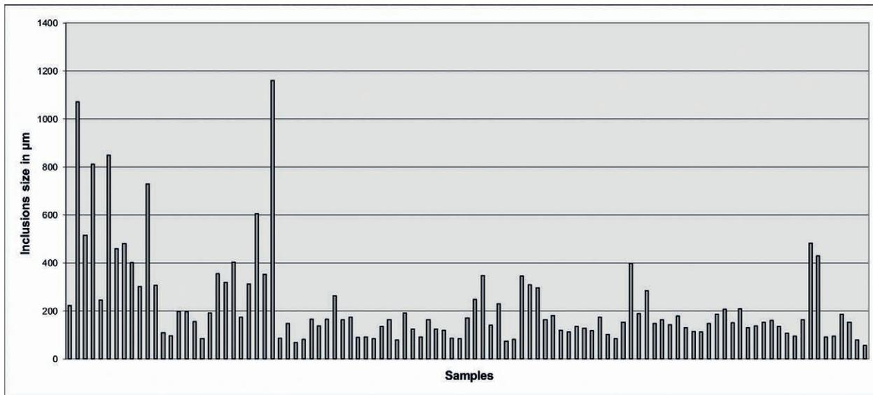
Fig. 16: Diagram showing the size of Cu-Fe sulphide inclusions in plate slags.
