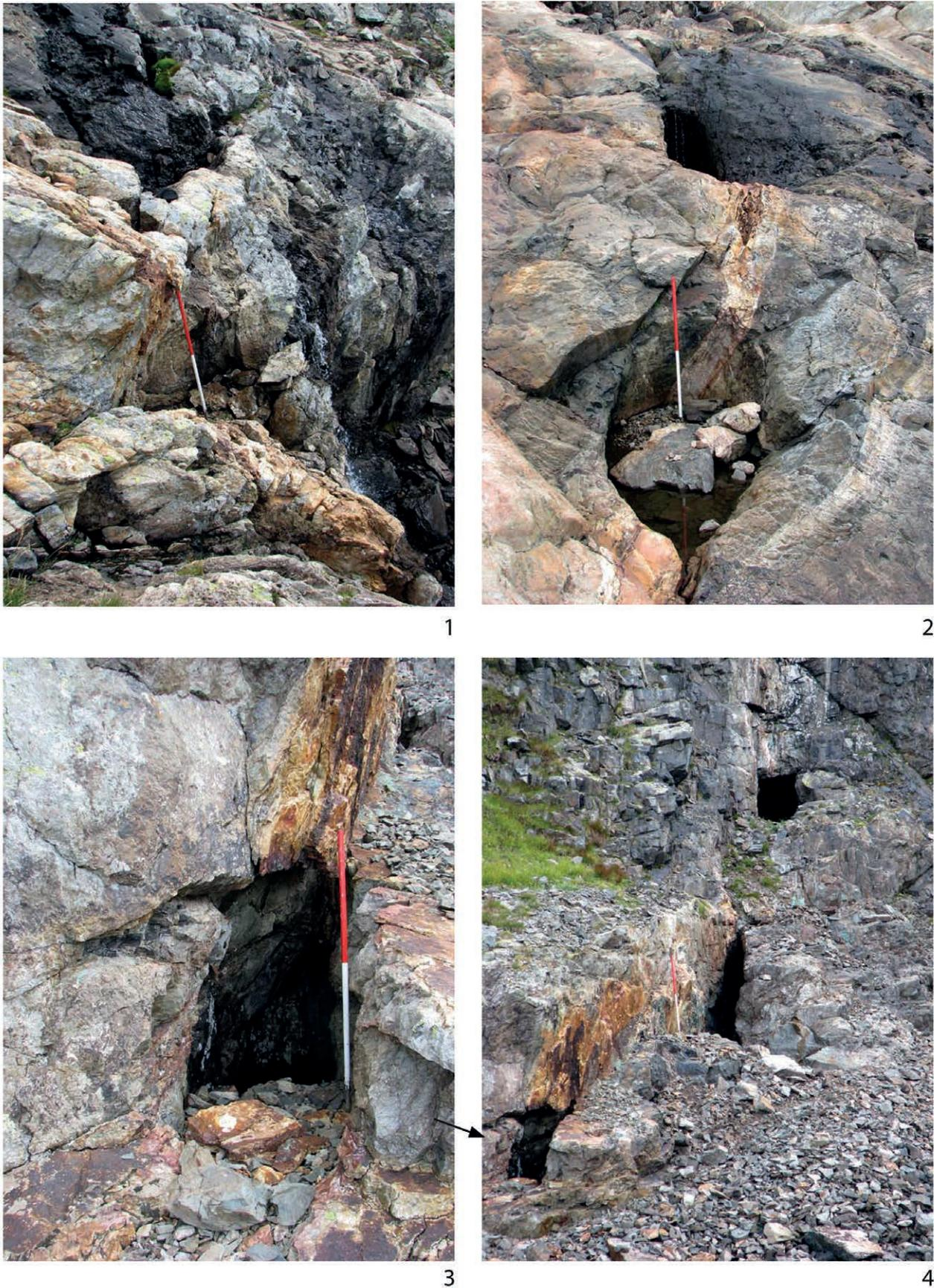
Fig. 11: Upper terrace of the Grandes Rousses, sector of Lac de La Fare (Isère): fire-settings and galleries for the extraction of copper ore. 1: no. 447, LF2, perched fire-setting on the right bank of a waterfall; 2: no. 448, LF2, two cupules stemming from fire-setting, currently flooded; 3: no. 454, LF1, refilled access to a gallery opened by fire-setting; 4: nos. 453 and 454, view of the three accesses of the gallery. The red and white stake measures 1 m in length.
