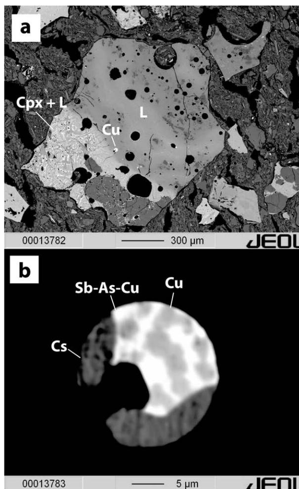
Fig. 9: Backscatter electron (BSE) images of a slag fragment from Kundl-Wimpissinger (sample W5). (a): slag fragment with the mineral assemblage clinopyroxene (Cpx) + glass (L). A small Cu-droplet is visible in the glass matrix. (b): close-up of the composite Cu-droplet showing a small-scale intergrowth between Cu and Sb-As-bearing Cu. The rim of the droplet is chalcosine (Cs).
