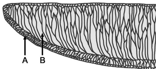
Fig. 24: Grain structure of a PCI: (A) Equiaxed grains and (B) columnar grains. Graphic adapted after a photo with the section of an experimental ingot cast into a drysand mould [see Tylecote, 1976, p.164, Fig. 1.3; University of Oxford, Research Laboratory for Archaeology and History of Art, Tyl\_316]; the top surface was exposed to air, while the bottom was at room temperature (graphic: D. Modl).
