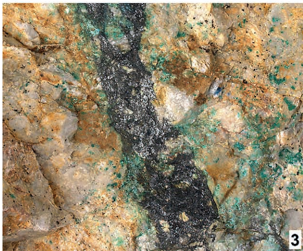
Fig. 2: Chalcopyrite from Mitterberg (1), fahlore in dolomite of the Late Bronze Age to Early Modern Age mine Mauk F, Radfeld, Tyrol (3); copper ore basis of northern alpine to southern bavarian copper and bronze findings (after Lutz & Pernicka, 2013) (2). (photo: DBM, M. Schicht, K. Stange, AVtention, Marienheide).
