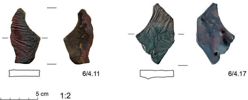
Fig. 9: Slag cake from the smelting site WH/SP 5 and plate slag from the smelting site WH/SP 4 (after Koch Waldner 2017; photos: A. Blaickner & T. Koch Waldner).
