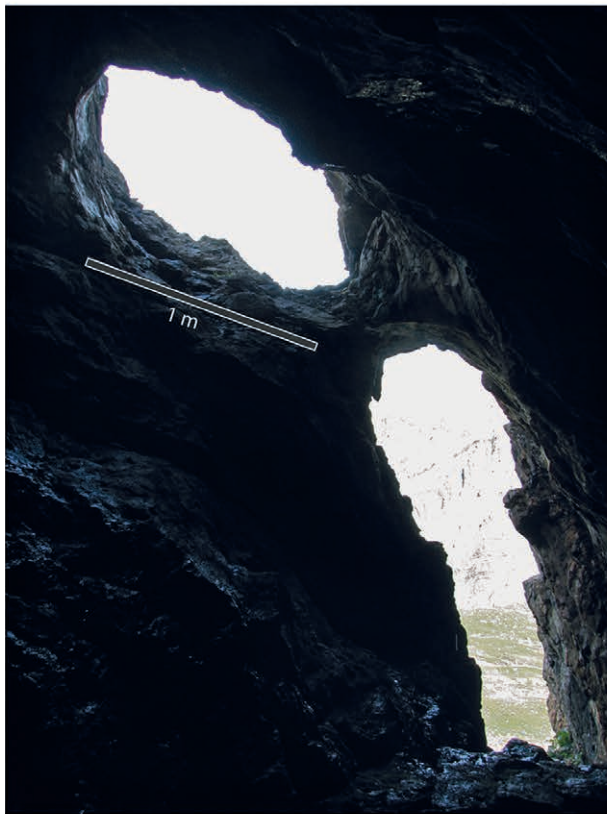
Fig. 10: Types of fire-settings. 1: working of a vein, notice the rubefaction of the quartz and its peel-like structure (Plan des Cavales); 2: vertical shaft on the vein (La Jasse 6); 3: gallery stemming from the connection of two workings, still marked by two accesses (Barbarate); 4: extraction trench produced by the coalescence of shafts and galleries (Plan des Cavales 4).
