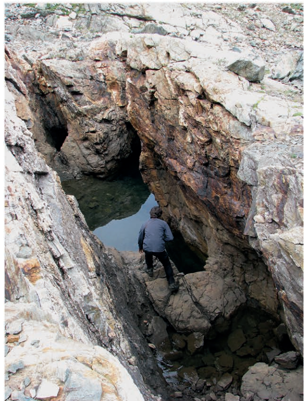
Fig. 10: Types of fire-settings. 1: working of a vein, notice the rubefaction of the quartz and its peel-like structure (Plan des Cavales); 2: vertical shaft on the vein (La Jasse 6); 3: gallery stemming from the connection of two workings, still marked by two accesses (Barbarate); 4: extraction trench produced by the coalescence of shafts and galleries (Plan des Cavales 4).
