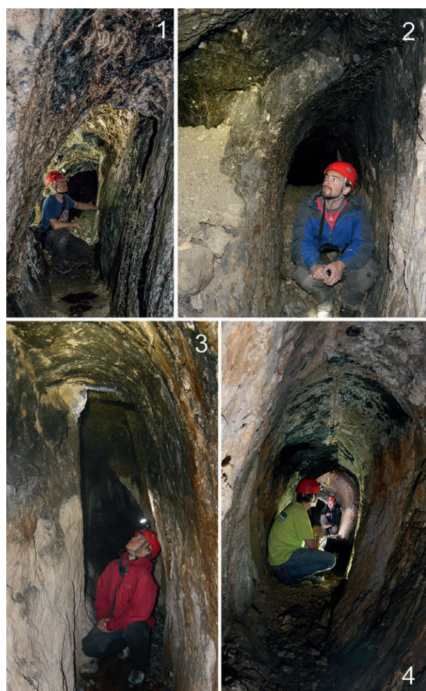
Fig. 19: Fire-set drifts from medieval/modern day mining activities: 1 - district Palleiten, 2 - district Weißer Schrofen, 3 - district Kleinkogel, 4 - district Hintersommerau (photos: M. Staudt and A. Schirmer).
