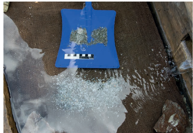
Fig. 14: A reciprocating 'pan' separation of chalcopryite from gangue within the water-filled box using just a flat-tipped hand shovel. Note the good retention of sulphide (photo: DBM).
