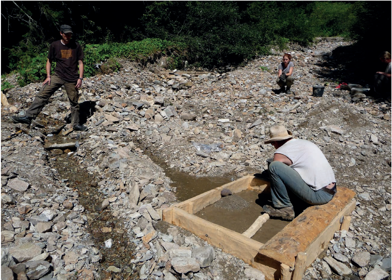
Fig. 4: Water-filled reconstructed box ready for experiments, showing lay-out of leat, diversionary channel and drain (photo: DBM).
