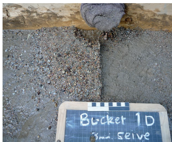
Fig. 7: Washed and partly separated chalcopyrite and gangue within the 'tye box' [Experiment 1d] (photo: S. Timberlake).
