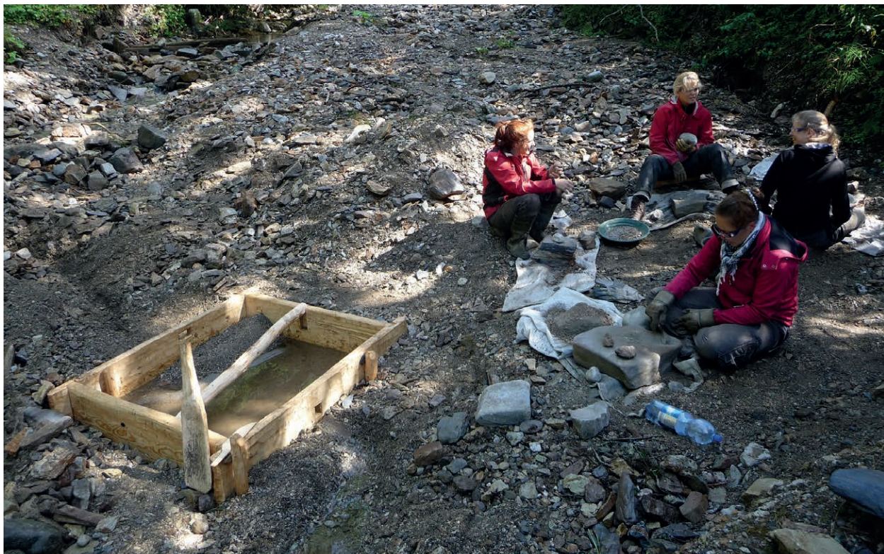
Fig. 3: 2012 river bed experimental ore-washing and processing site, Mitterberg (photo: S. Timberlake).
