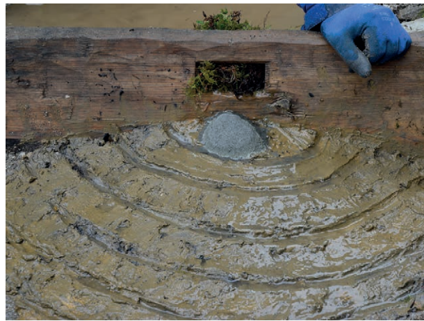
Fig. 10: Tye box experiment in August 2016 using the clay cone and sphagnum moss as a ‘bung’ to control water inflow (photo: DBM).
