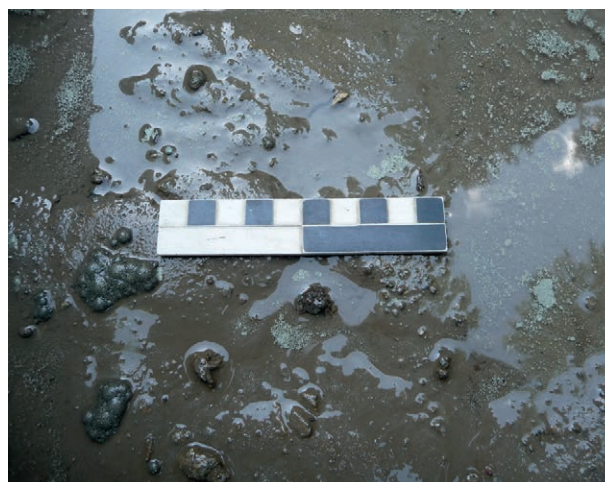
Fig. 8: Flotation of fine chalcopyrite bubbles upon the water surface. August 2012 experiment (photo: S. Timberlake).
