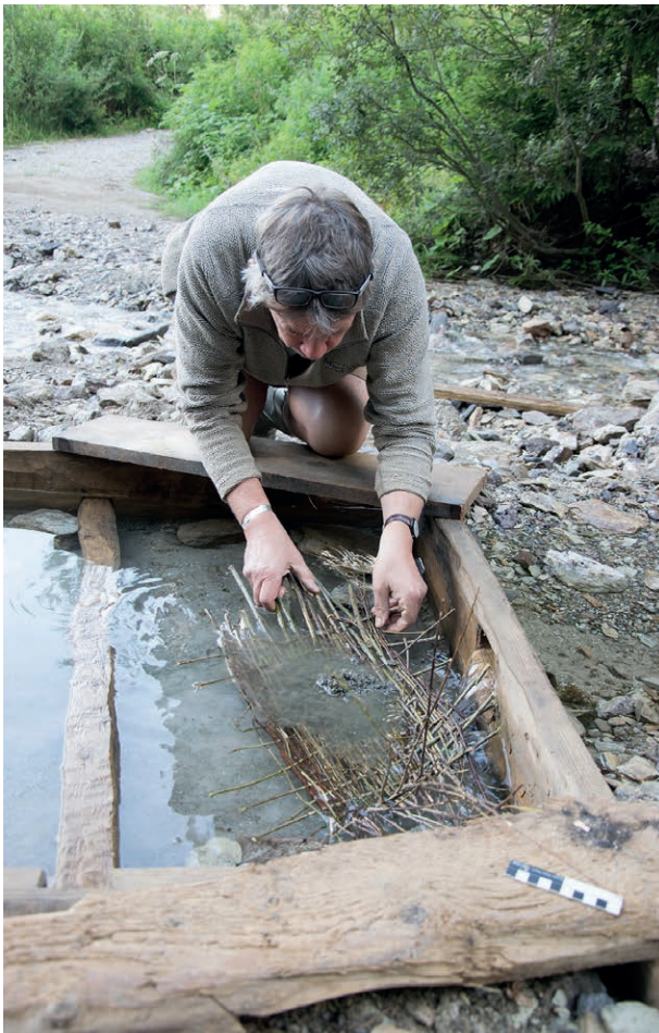
Fig. 12: Experiment 3.1 or 3.2 in August 2016 Using an open weave withy sieve ( Corylus or Salix ) in an attempt to jig separate good ore from gangue within the water-filled tank (photo: DBM).
