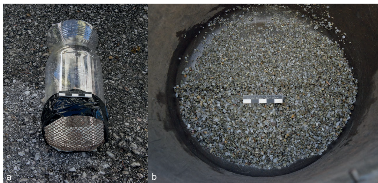
Fig. 11a + b: The 'mini-jig' sieve container used to test the principle of jig separation of the chalcopyrite (sulphide fraction) from the lighter quartz-rich gangue. Figure 11b shows this gangue fraction in the sieve with about 25% of the chalcopyrite remaining (photo: DBM).
