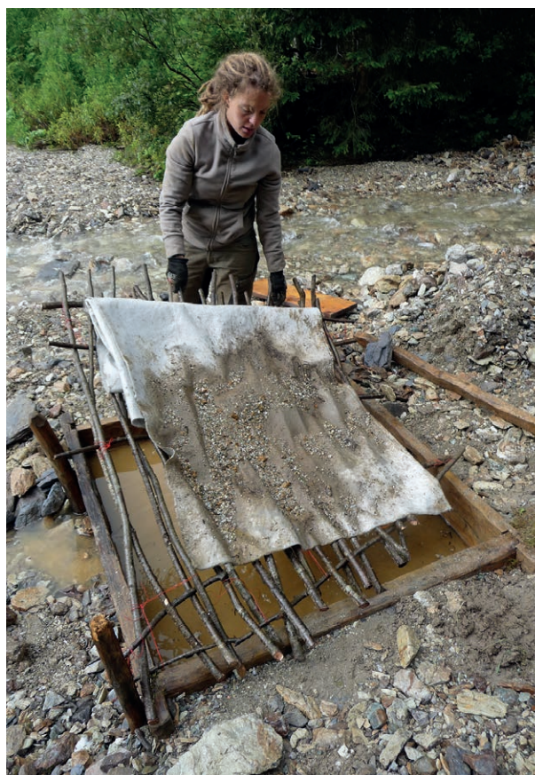
Fig. 9: Using the water-filled box with a woven wattle frame and sacking for the washing of the crushed ore in August 2016 (photo: S. Timberlake).
