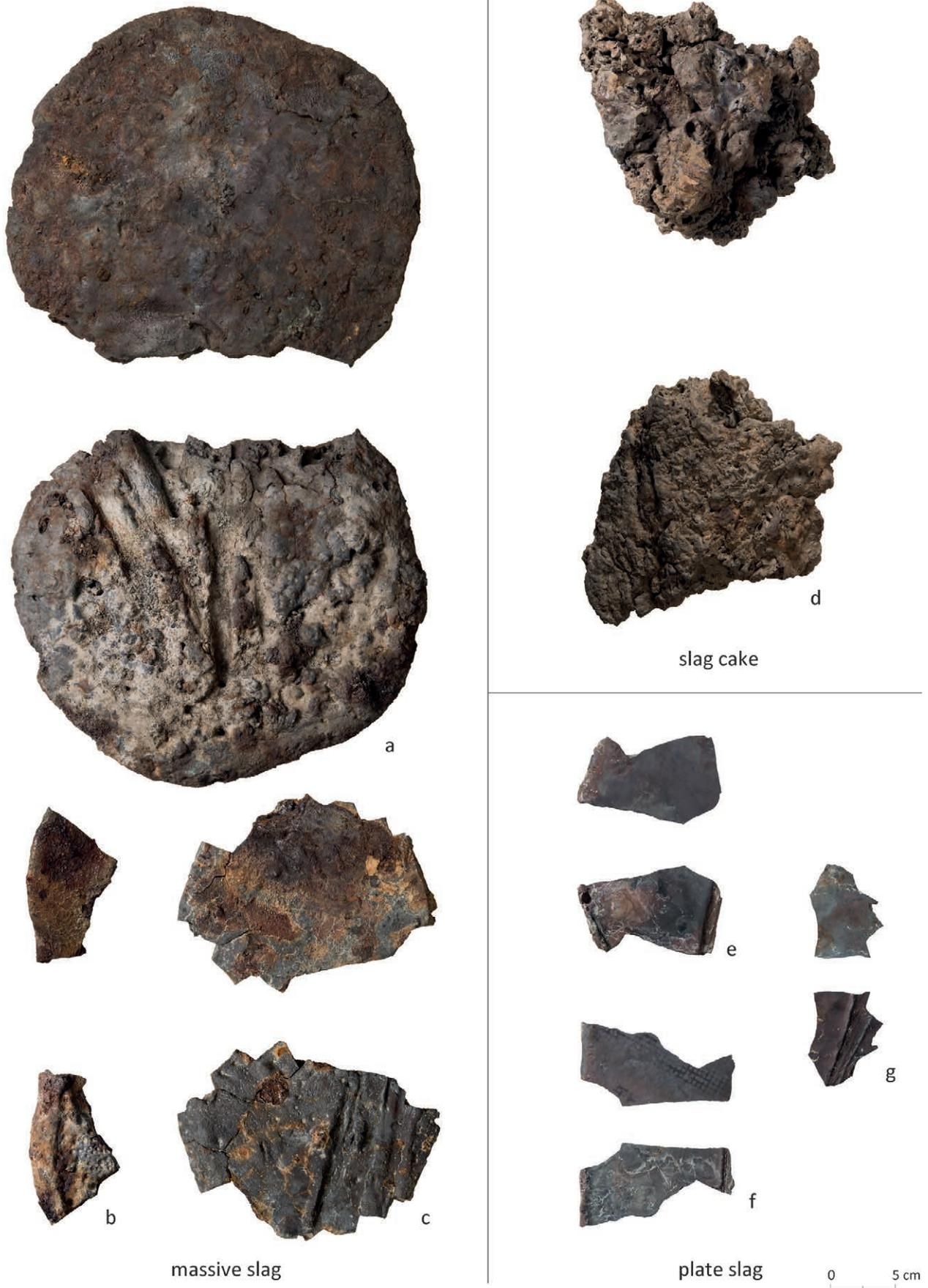
Fig. 3: The surface colour changes are due to strong corrosion (a-c) and surface reactions during the drying process on a metal lattice (f). (Ill./photo: Archaeological Service of the Canton of Grisons).
