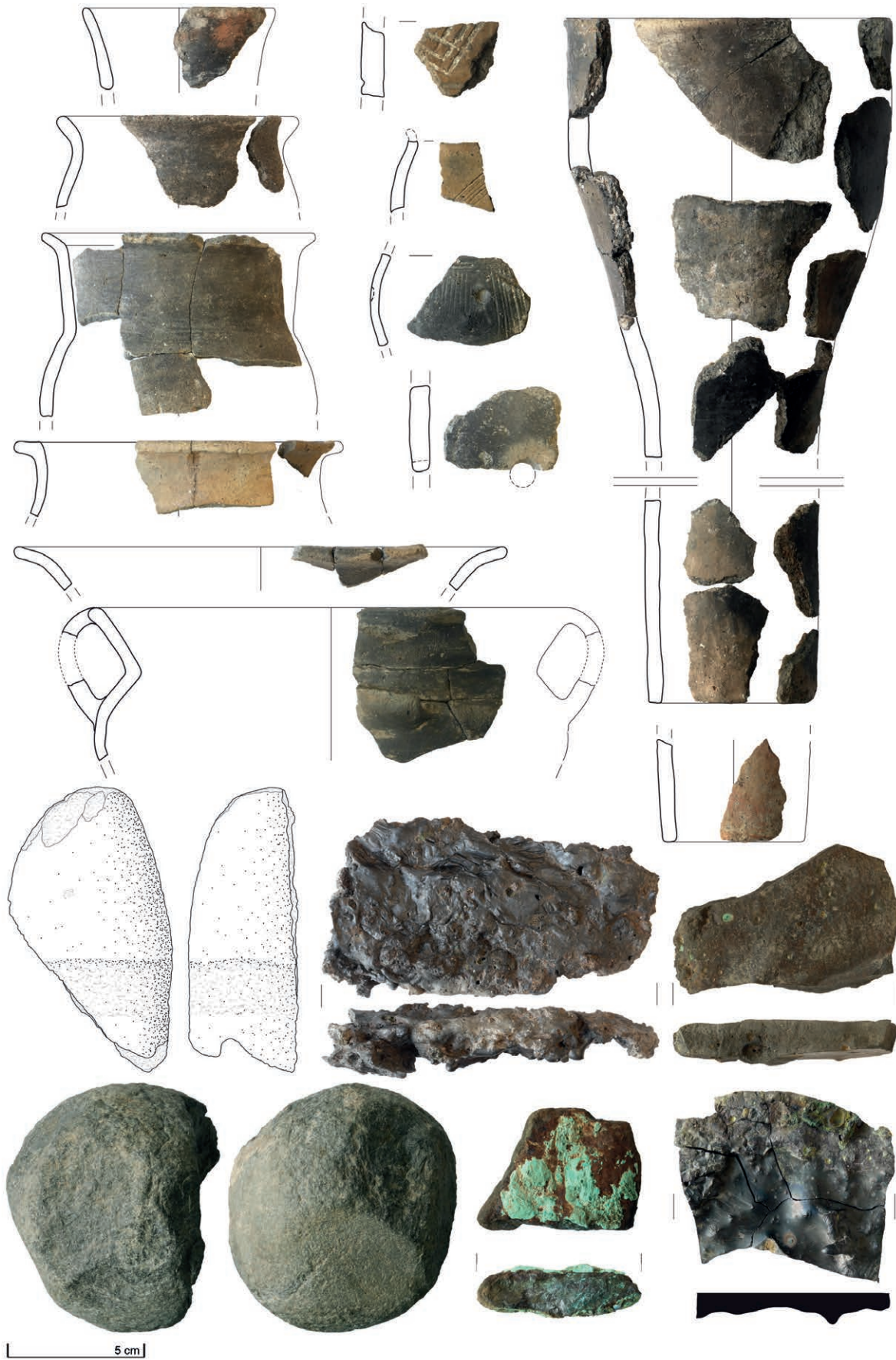
Fig. 13: Finds from the smelting site Rotholz: plate slag (RH8_10, RH20-2_16), heterogeneous slag (RH7-2_15), fahllore (RH13-2_15), fine ceramics (RH4-3_16, RH14-3_15, RH17-16_16, RH17-18_16, RH28_16, RH30_17, RH35-2_17, RH43-2_17), encrusted domestic pottery (RH25_16), fragments of tuyères (RH10_17, RH10-6_17, RH17-20_16) and stone tools (RH3_10, RH31_16; graphics: M. Staudt).
