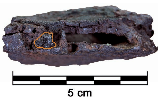
Fig. 22: Fragmented PCI with a good visible slag grain and a elongated gas cavity on the fracture surface; single find (see Windholz-Konrad, 2003, p.93, 127, cat.no.534, fig.124) from finding area 'Obertraun-Traunweg' near Hallstatt, Upper Austria (photo: D. Modl).
