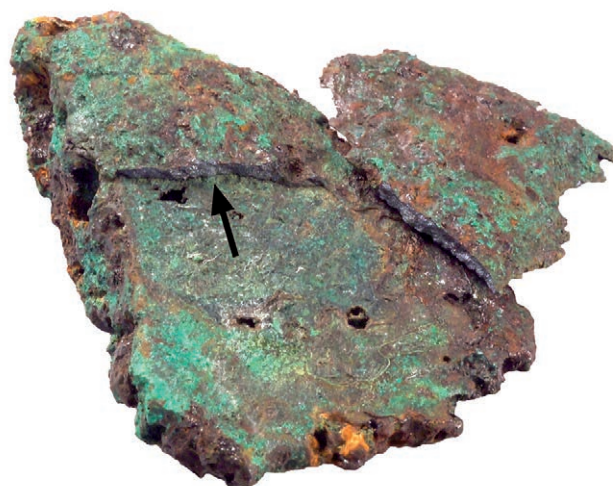
Fig. 28: PCI fragment (presumably base-metal speiss with 60,76 wt% Cu, 15,13 wt% As, 0,36 wt% Ni, 13,91 wt% Fe) with an adherent, silvery metallic phase on the top side (80,50 wt% Cu, 0,93 wt% As, 0,03 wt% Ni, 15,44 wt% Fe) from the so-called Brandgraben hoard (CNr. 15; Bz D/Ha A1/A2-Ha B3; see Windholz-Konrad, 2018, p.46, 60, Fig. 34/189) near Bad Aussee, Styria (photo: D. Modl).
