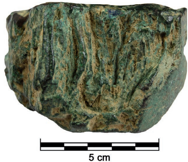
Fig. 25: Fragmented PCI with good visible columnar grains and hammer marks on the fracture surfaces from a hoard (HaA1) near Lannach, southwest of Graz, Styria (photo: D. Modl).
