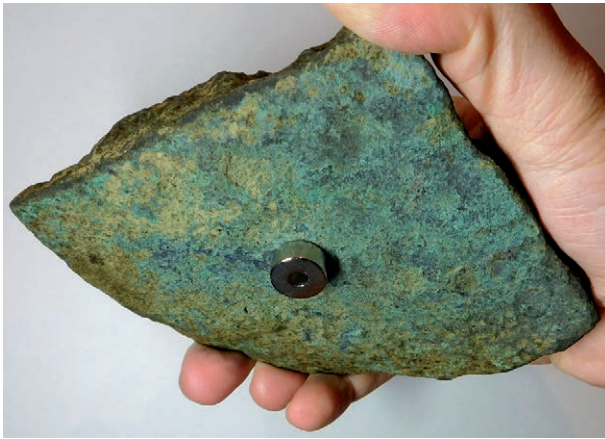
Fig. 15: Ferrous PCI with an adhere neodymium magnet ring (N35) (photo: D. Modl).
