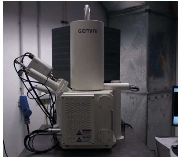
Figure 6.2 Scanning electron microscope with energy dispersive spectroscopy capabilities at the Deutsches Bergbau-Museum Bochum (Photo: S. Merkel 2012).
