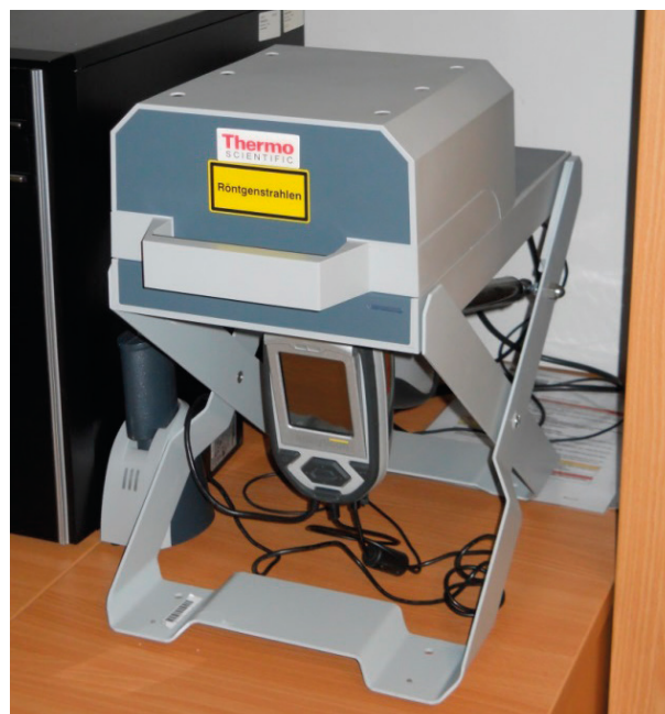
Figure 6.3 Portable X-ray fluorescence device docked to a protective sample chamber, Deutsches Bergbau-Museum Bochum (Photo: S. Merkel 2012).
