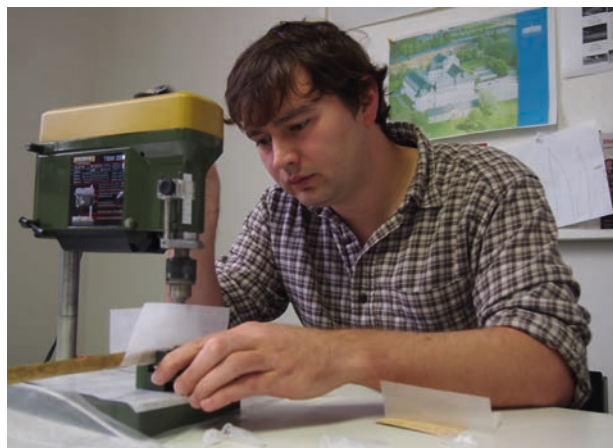
Figure 6.4 Taking samples of metallic objects with portable drill press at Schloss Gottorf (Photo: V. Hilberg 2013).
