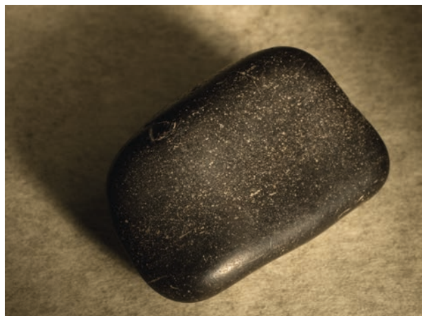
Figure 2.4 Touchstone from Hedeby (MAIXNER 2010, Figure 30) 4.4 cm x 2.9 cm x 1.2 cm. Such stones were used to examine the streak of precious metals to interpret the composition.
