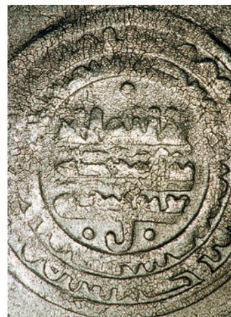
Figures 5.4 and 5.5 Samanid double dirham minted at Panjīr, Aghanistan under Nuh I. ibn Nasr, 942-954 AD (331-343 AH) (STÖLLNER et al. 2004, 804, Cat. 536). This dirham exhibits cracking due to the brittleness of the silver, and this is characteristic of high bismuth silver. The composition of the coin is recorded as 87% silver, 2.5% copper, and the remaining 10.5% probably consists of bismuth and lead: the values were not provided.
