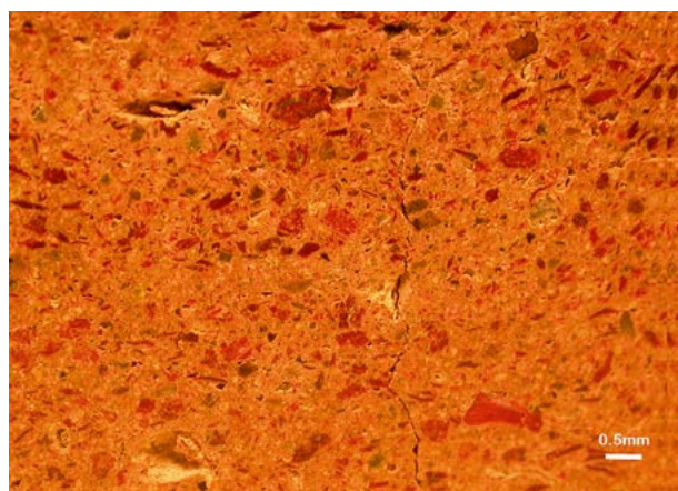
Fig. 11: Optical micrograph of the material of the cupel of Fig. 8, showing a kind of breccia microstructure characteristic of material produced by a mortar. It consists of angular fragments of broken litharge embedded in a fine-grained matrix. (Optical micrograph: G.D. Papadimitriou).
