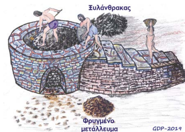
Fig. 5: Schematic representation of a roasting furnace during the charging phase with galena and a small proportion of charcoal. (Drawing: G.D. Papadimitriou).
