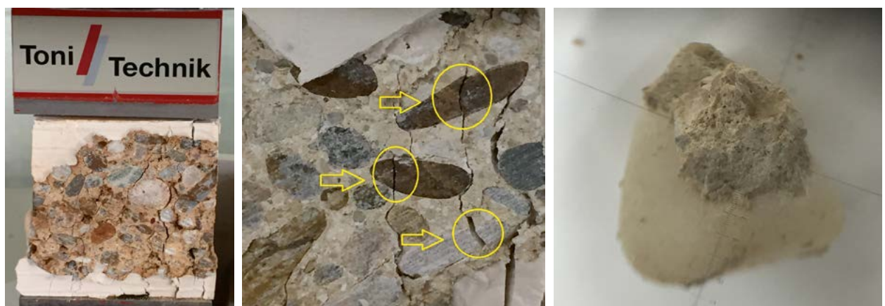
Fig. 10: (a) Assessment of compressive strength (b) Cracks deviating through aggregates during compressive strength testing, (c) High adhesive strength between binder and aggregates (photos: N. Meimaroglou).
