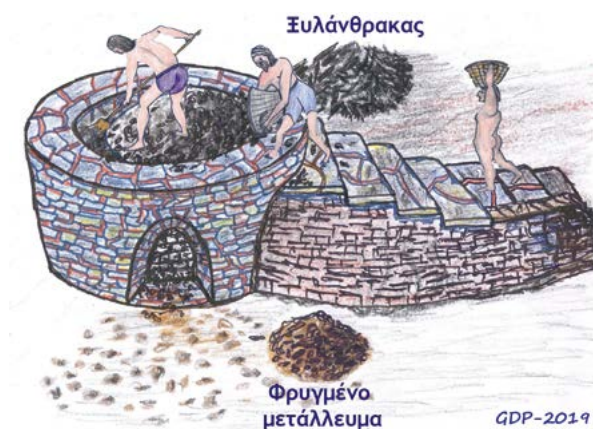
Fig. 5: Schematic representation of a roasting furnace during the charging phase with galena and a small proportion of charcoal. (Drawing: G.D. Papadimitriou).
