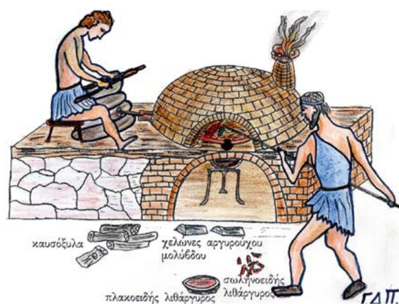
Fig. 6: Virtual reconstruction of a cupellation furnace of the classical period at Laurion. (Drawing: G.D. Papadimitriou).
