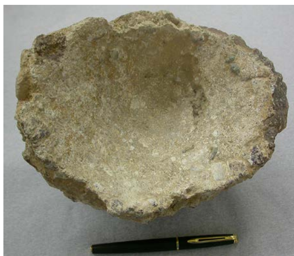
Fig. 8: Deep Cupel of conical form from Megala Pefka (Legrena, Laurion), Classical to Hellenistic period. (Photo: G.D. Papadimitriou).
